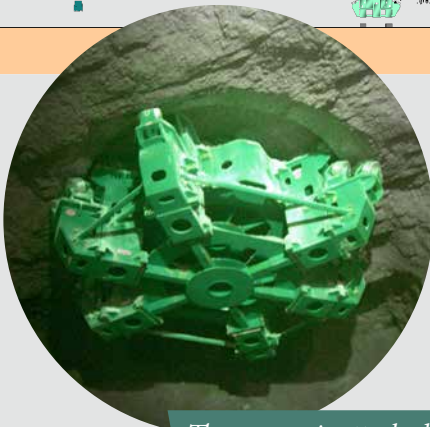
The reamer is attached and bores upwards through the rock.
